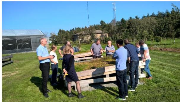
*Discussion concerning the green roofs (10 pieces: 2 x 3 meters) at the seminar hosted by Nibio Særheim in September 2016. Each roof can easily be replaced and each unit is therefore a test station for runoff and other performance characteristics.*
